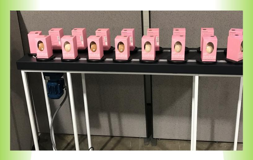
Special 91.5-inch straight conveyor. This double-sided conveyor comes with an optional support stand. The dimensions of the unit:
